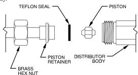
Fig. 16 – Refrigerant Flow-Control Device
