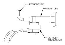
Fig. 7 – Defrost Thermostat Location
