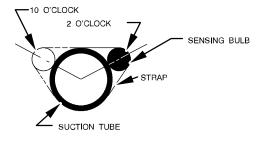
Fig. 15 – Position of Sensing Bulb
