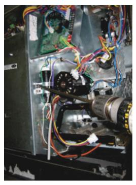
Fig. 32 – Removing Mounting Screw from Gas Manifold  $^{\rm A210076}$
