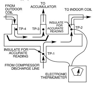
Fig. 13 – Reversing Valve (Heating Mode, Solenoid De-Energized)
