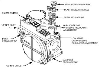
Fig. 40 – Two-Stage Gas Valve (208/230 VAC Models)
