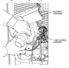
Fig. 36 – Removing Inducer Assembly
