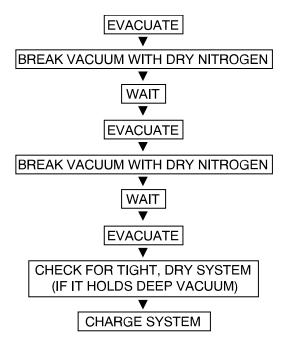
Fig. 20 – Triple Evacuation Method
