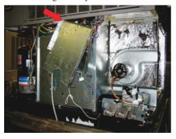
Fig. 35 – Securing Assembly to Screw Hole
