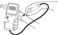
Fig. 17 - Electronic Leak Detection
