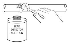
Fig. 18 - Bubble Leak Detection
