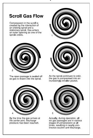
Fig. 10 – Scroll Compressor Refrigerant Flow
