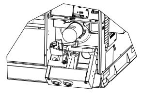
Fig. 44 – Burner Rack Removed (Standard and Standard Low  $\overset{A07680}{NOx}$ **Models Only)**
