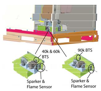
$\label{eq:Fig.31-Burner Thermal Switch (BTS) (Ultra Low NOx)} \textbf{NOx} \\ \textbf{Inducer Draft Blower Assembly Removal}$
