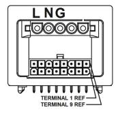
Fig. 26 – EON<sup>TM</sup> Module Plug (Advanced Dehumidification Models)
