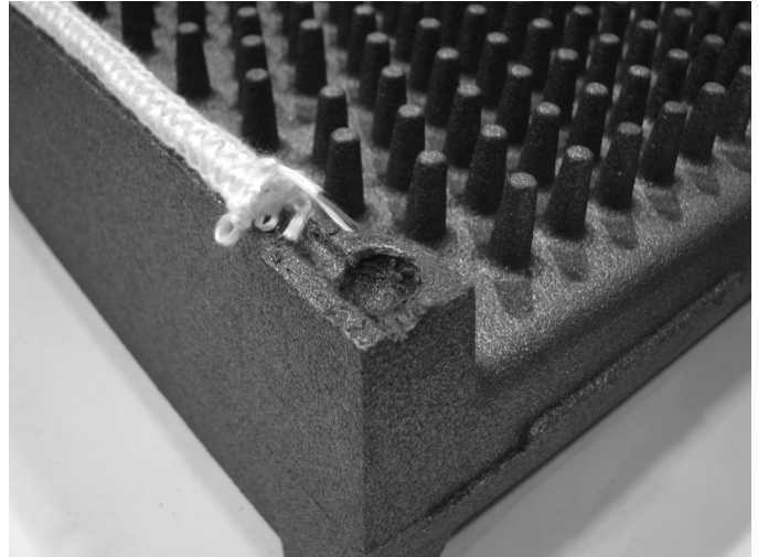
Figure 4a Corner after exposed silicone has been removed.
