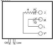
Fig. 4 — P45NAA, single voltage \*V: 120 VAC, 208 VAC, 240 VAC or 24 VAC
