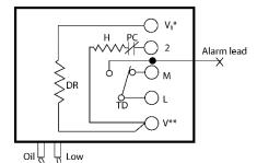
Fig. 6 — P45NCB, dual voltage with alarm circuit
