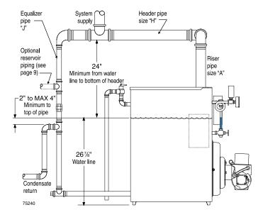
Figure 7 Recommended piping, OSB-3, -4 and -5, piping for parallel-flow systems only
