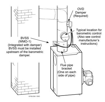
OVD Vent damper kit Part Number 381-800-515WT must be installed in all installations. The vent damper is supplied with the boiler. Refer to the damper instruction manual and to Figures 3 and 4 for damper location. A blocked vent shutoff switch (BVSS) is integrated into the damper wiring harness.
