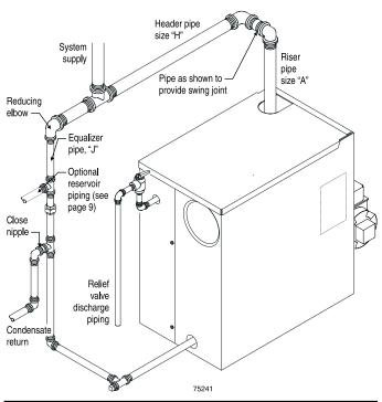
Figure 8 Recommended piping, OSB-6, piping for parallel-flow systems only
