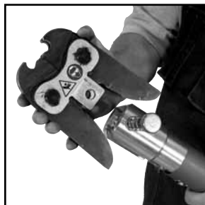
Figure 7: Placement of adapter jaw into the tool
