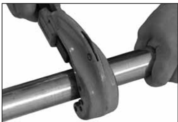
Figure 1 — Cut tube to desired length using a tube cutter
