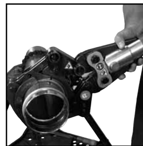
Figure 8: Placement of adapter jaw into pressing chain
