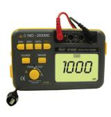
The Versatile M1000D Provides the User Selectable Test Voltage Ranges of 250V/500V/1000V to Test Insulation Resistance and Can Also be Used to Measure AC Voltage up to 750AC.
