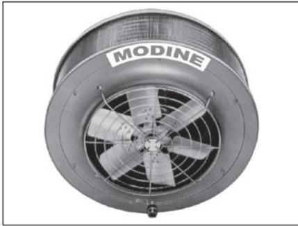
Vertical delivery unit heaters are ideal for heating buildings with high ceilings or areas that require the heater to be mounted above obstructions such as craneways. Selection from a variety of heat throw patterns is made easy by choosing from four types of air deflectors. Heat throw patterns range from a high-velocity narrow jet to a gentle-velocity broad based cone of heated air.
