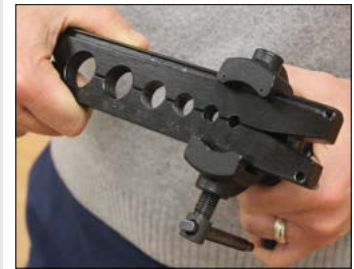
Railing allows yoke to smoothly travel while keeping the flaring tool and bar aligned
