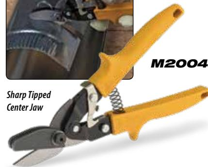
**The Max2000 Double Cut Snip** employs a best of all worlds close tolerance design for consistent performance. A curved cutting edge on the center jaw reduces cutting force required and large relief grinds on all jaws minimize drag. The double cut blades feed smoothly, cut cleanly without surface distortion, and easily navigate metal seams encountered in round metal duct and stove pipe. A self-starting point on center jaw makes short work of blind cuts.
