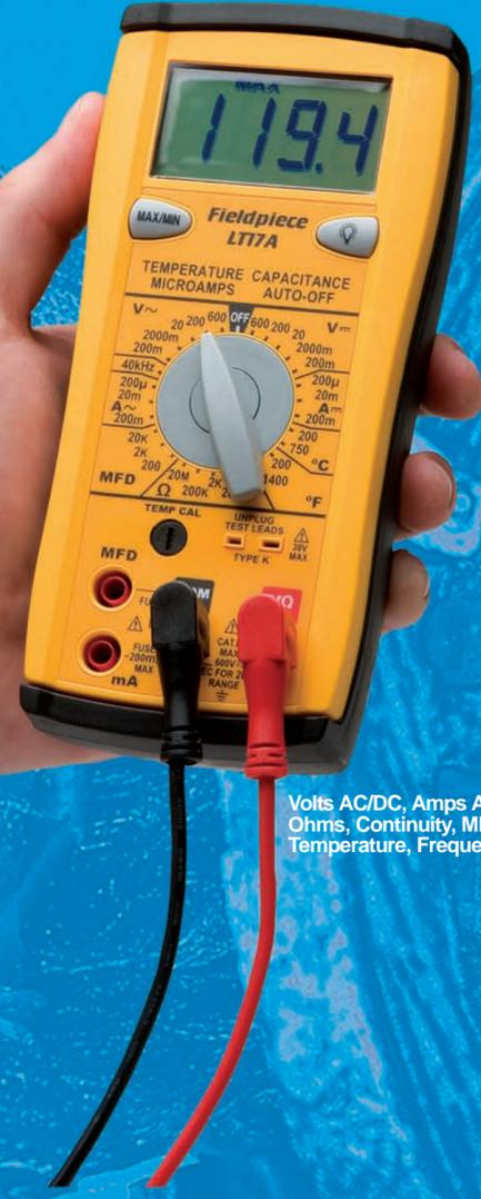
Volts AC/DC, Amps AC/DC, Ohms, Continuity, MFD, Temperature, Frequency
