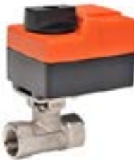
2-Way, Characterized Control Valve B214B, TR24-3-T US This valve is typically used in air handling units on heating or cooling coils, and fan coil unit heating or cooling coils. Some other common applications include Unit Ventilators, VAV box re-heat coils and bypass loops.
