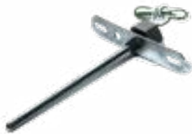
Discharge Air Sensor ZPA-DTS The ZPA-DTS is a duct-mounted temperature probe that provides capacity control of heating and cooling equipment. It senses the delivered air temperature and cuts off the heating or cooling when the delivered air temperature goes above or below normal operating limits.
