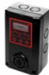
Toxic & Combustible Sensors Q5-CO-250P-0-X, Q5-NO2-10P-0-X The Q5 Series is a microprocessor based "smart" gas transmitter. It is paired with either an electrochemical gas sensor for toxic gases, or a catalytic bead sensor for combustible gases.
