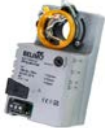
Replacement Damper Actuator FP18-Motor Belimo 24V, 60 second, 18 in-lb Actuator
