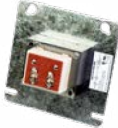
40VA Transformer TR-40 120V Primary 24V Secondary 40VA Transformer Box mounted and multi-tap also available TR-40-B, TR-40-MT
