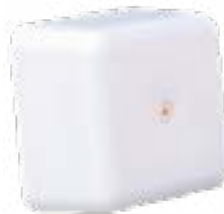
Outdoor Temperature Sensor ZPA-OTS The ZPA-OTS is installed in the heat pump unit when backup heat is being used. This outdoor temperature sensor detects the ambient temperature, directing the zoning panel when to switch to the auxiliary heat source.
