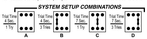
**IMPORTANT**: It is best to remove the jumpers before installing the **ICM283**. <u>Do not</u> cut the jumpers with power applied to the control. Completely remove unneeded jumpers. Carefully cut the jumper with wire cutters and discard the jumper.
