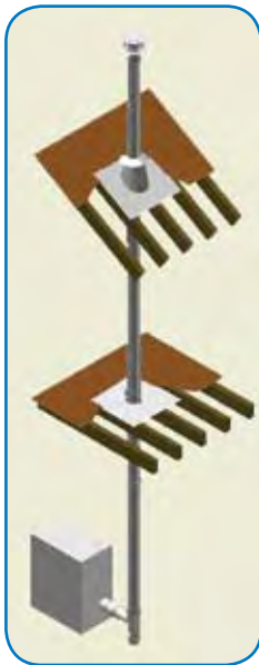
FasNSeal® Vertical - Through the roof installation
