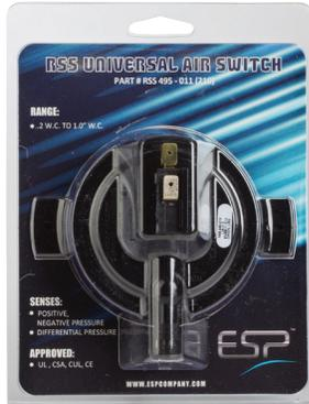
Series RSS-495-11 Air Sensing Switch Kit contains compact, economical switches designed for a residential furnace and light commercial aftermarket applications. The RSS-495 switches have an adjustable set point range of 0.25" W.C. to 1.0" W.C. (they have been factory set to activate on a pressure rise of 0.25" W.C.). The field adjustability makes these switches ideal for aftermarket residential furnace applications, electronic air cleaners and humidifiers.
