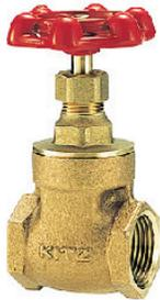
Forged Brass Gate Valves have screwed-in-bonnet, non-rising stem, solid wedge disc, integral seat, NPT threaded or solder joint ends
