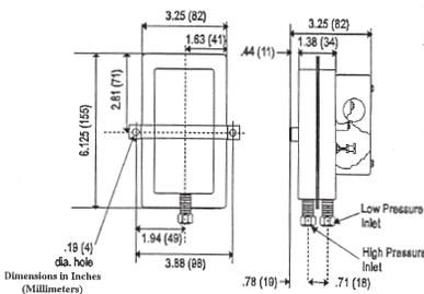
The model AFS-262 is a general purpose proving switch designed for HVAC and Energy Management applications. It may be used to sense positive, negative, or differential air pressure. Installation kit included.
