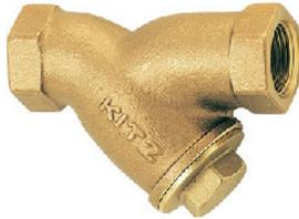
Y-Pattern Strainers provide protection for equipment having internal moving parts. Has blow-out outlet for easy clean-out, threaded cap for easy removal. Bronze body and Type 304 stainless steel screen. NPT threaded ends or solder joint ends.
