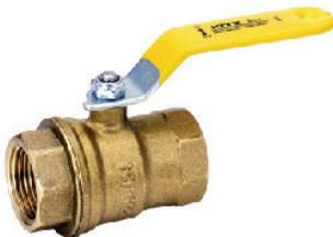
Full Port Brass Ball Valves are two-piece construction with a chrome plated brass ball, blowout-proof stem, PTFE seats and double ‘O’ ring stem seal. Quick quarter-turn for easy operation. For use in plumbing and light industry applications. Standard NPT end connection.
