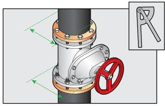
Using divider, draw inner and outer circumferences on two separate pieces of AEROFLEX Sheet.
