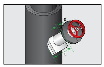
Transfer measurement of 1/2 ring circumference (1/2 c) and inner/outer strainer dimensions to AEROFLEX Sheet of the same thickness.
