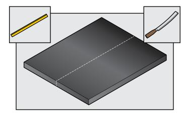
Apply AEROFLEX adhesive to cut edges of longitudinal seam, allow to tack up until ready for contact.
