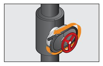
On AEROFLEX Sheet (same thickness), lay circumferential strip on sheet and mark into 4 equal segments.
