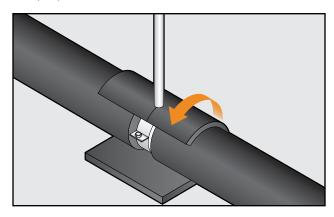
Seal all fitting cover seams and to outer surface of adjoining tubes with AEROFLEX adhesive to provide complete vapor seal.
