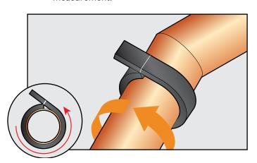
Measure the inner height (X) and out height (Y) of miter joint.
