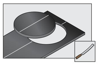
Apply Aeroseal adhesive to both surfaces and allow to tack.
