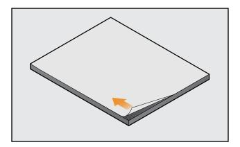
Position and align exposed edge at termination or transverse edge.
