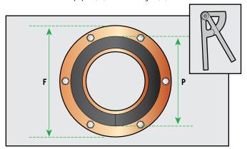
Using divider, draw inner and outer circumferences on two separate pieces of AEROFLEX Sheet.
