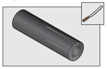
Glue notched edges together with AEROFLEX adhesive
