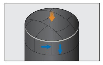
Once all sections of the dome are insulated, glue perimeter seam with Aeroseal adhesive under compression to create vapor seal.
