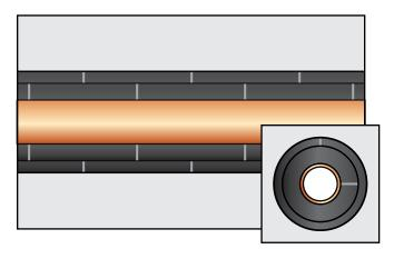
Glue butt joints under compression with AEROFLEX adhesive.
