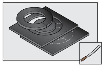
Wrap rings around pipes on both sides of flange and fully adhere to insulation inserts and bolts with AEROFLEX adhesive; do not glue rings to installed pipe insulation yet.
