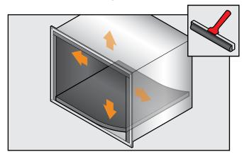
• Ensure that all four (4) inside corner edge seams fit under compression with no gaps present since it is impractical to seal them with adhesive.
