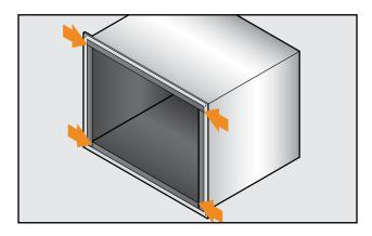
Seal all transverse edges under compression with Aeroseal or Aeroseal LVOC Black adhesive.
