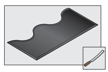
Apply AEROFLEX adhesive to longitudinal seam, allow to tack and seal around spindle housing.
