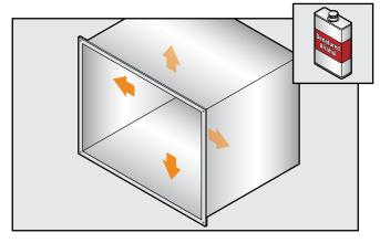
Measure duct dimensions and cut AEROFLEX Sheet & Roll with straight edge.
