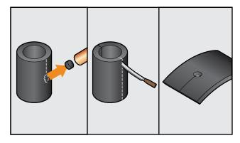
Wrap fitting cover over hanger and check for proper fit (do not stretch).
