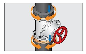
Measure circumference of rings (C) with strip of AEROFLEX Sheet that is the same thickness (do not stretch); add 1/4" [.64 cm] to measurement.
