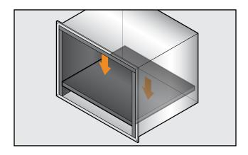
• To remove PSA release liner, pinch corner of sheet/roll and peel back 1"-2" [2.5 cm - 5 cm].
