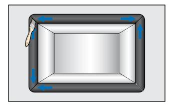
Wrap flange cover around duct flange and glue final 45° seam.
