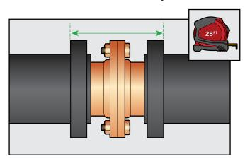
Draw with straight edge and cut flange jacket from AEROFLEX Sheet.
