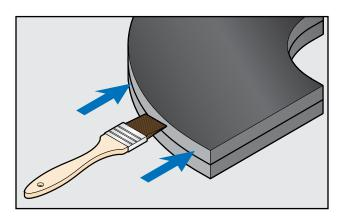
Once glued edges are ready for contact, adhere outside edges together from the outer edges inwards.
