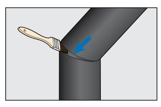
When ready for contact, join longitudinal seam first followed by miter seam with firm pressure under compression.
