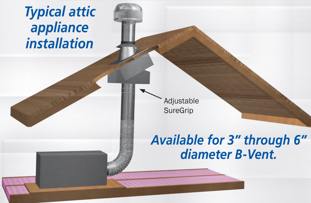
Continue adding pipe sections – supports up to 90 lbs.
