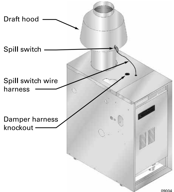
Figure 7 Spill switch with wire harness
