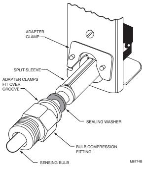
Fig. 7. Direct immersion model with fitting partially removed.
