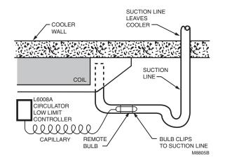
Fig. 17. Attaching remote bulb to horizontal suction line.
