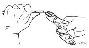
Fig. 13. Removing excess bulb support.
