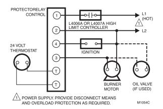
Fig. 20. Typical oil-fired gravity system.
