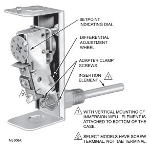
Fig. 6. Internal view of L6006A.
