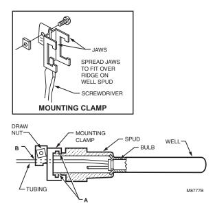
Fig. 8. Immersion well fitting.
