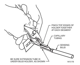
Fig. 14. Securing capillary in bulb holder.
