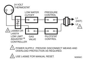
Fig. 19. Typical gas-fired system with domestic hot water.
