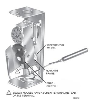
Fig. 31. Adjusting the differential.
