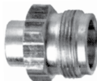
G492 1/4" FPT x male 1"20 thread w/"O" ring. No check valve.
