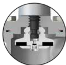
Integrated Back Check Feature
