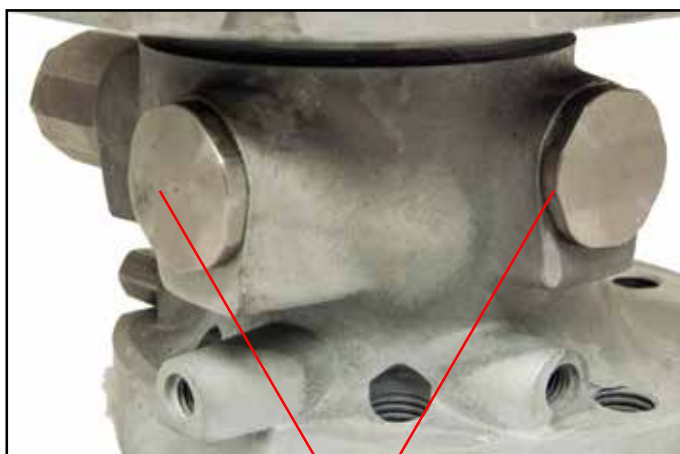
Alternate Gland Ports (Plugged)
