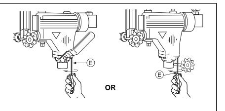
f. Remove the blow down valve (D) from the control (A). If necessary, use a hammer to tap it loose.
