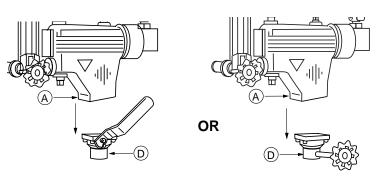
NOTE: For spring type blow down valves, the spring mechanism must be removed from the control body.
