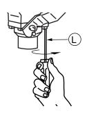
**e.** Verify that the blow down valve (H) is unobstructed by opening and closing the valve over its full range of motion (90°).
