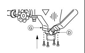
**d.** Using a flathead screwdriver (L), tighten the screws to approximately 15 ft•lb (20 N•m).
