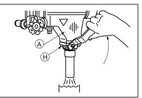
g. Close the blow down valve (H) and check for leakage by following the instructions in "Step 3" section e.
