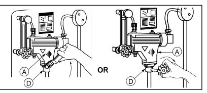
**d.** Using a pipe wrench (B), remove the blow down pipe (C) from the existing blow down valve (D).
