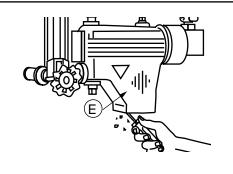
h. Using a scraper, remove the old gasket (F) from the control (A). The gasket sealing surface (G) must be smooth and clean for proper installation.
