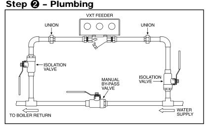
Feeder must be installed with a manual by-pass. Use isolation valves and unions to allow easy removal for service or replacement. Note: Arrow on VXT valve indicates direction of water flow.
