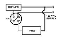
d. Connect the wire from the burner to terminal #1 of the low water cut-off. Connect a "jumper" from terminal #2 to terminal #3 of the low water cut-off. Connect a wire from terminal #4 of the low water cut-off to the remaining wire in the 101A water feeder.
