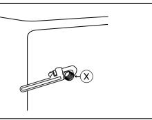
b. Install the control (A) by rotating it onto the 2½" (63.5mm) nipple (X, as shown in Step a on previous page). Tighten to 109 ft•lb (148 N•m).
