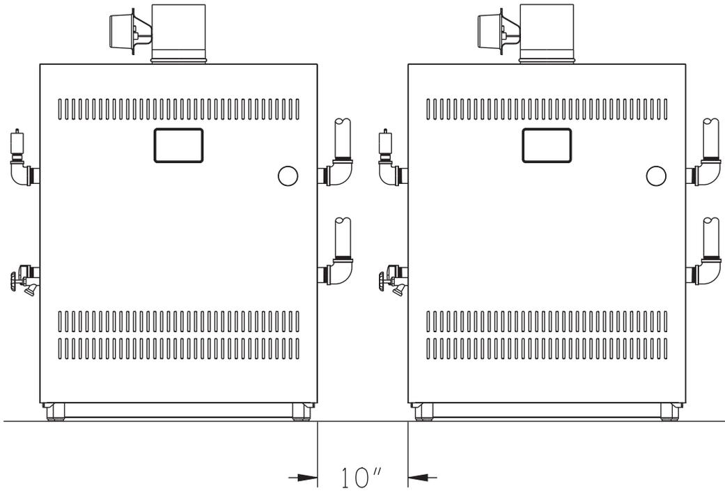
FIGURE 2.2: ALTERNATE REDUCED CLEARANCE BETWEEN BOILERS
