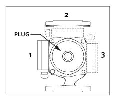
Do not hang items or articles of clothing on the pump as air must be able to circulate freely through the motor. Do not operate the circulator without the motor plug installed.
