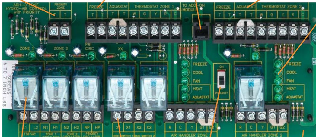
Premium Plug-In Replaceable Relays for long life. High relay load rating 10A.
