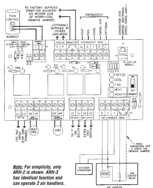
When used with Indirect Hot Water Heaters, priority feature allows all hot water circulation to stop except for priority zone.
