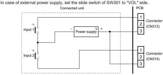
\*1: The switches can be used on the following condition: DC 12 V to 24 V, 1 mA to 15 mA. \*2: Make the power supply DC 12 to 24 V, 10 mA or more.
