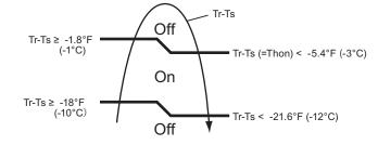
Tr: Room temperature Ts: Set temperature Thon: Heater on temperature
