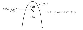
Tr: Room temperature Ts: Set temperature Thon: Heater on temperature
