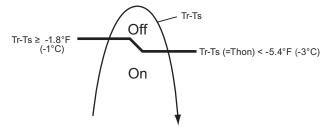
Tr: Room temperature Ts: Set temperature Thon: Heater on temperature
