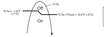
Tr: Room temperature Ts: Set temperature Thon: Heater on temperature
