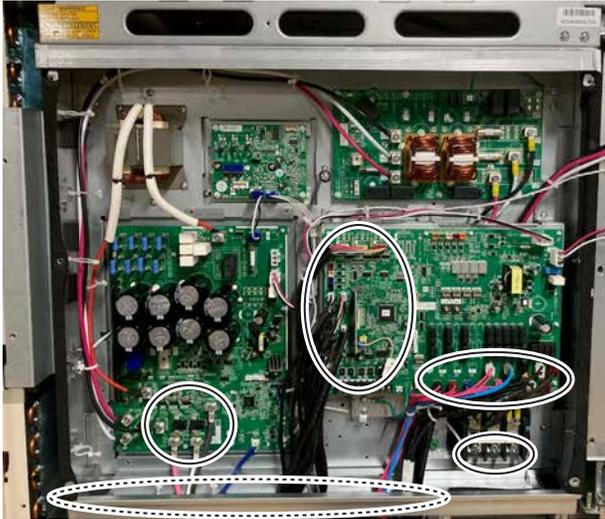
1. Remove the connectors, cables, 3 mounting screws, power cable, transmission cable and cable ties.
