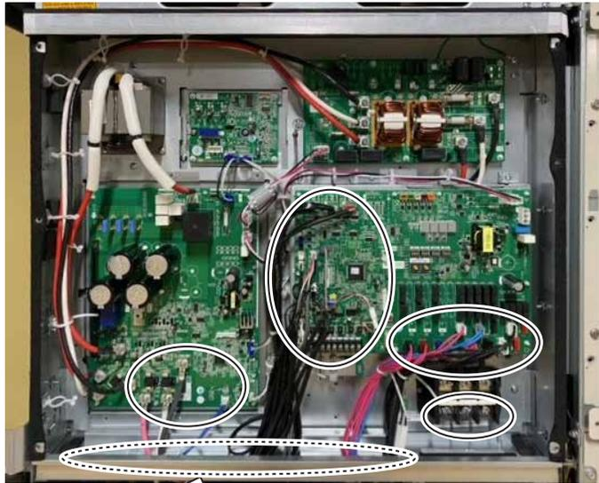
1. Remove the connectors, cables, 3 mounting screws, power cable, transmission cable and cable ties.
