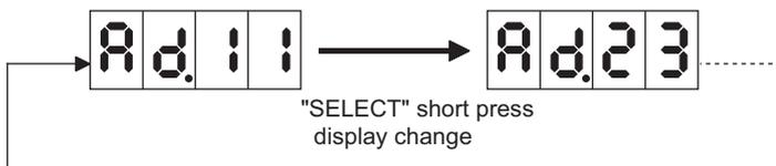
\* Only in the case of “indoor unit abnormal (E.5U.1)”, indoor unit address is shown by ENTER long press.
