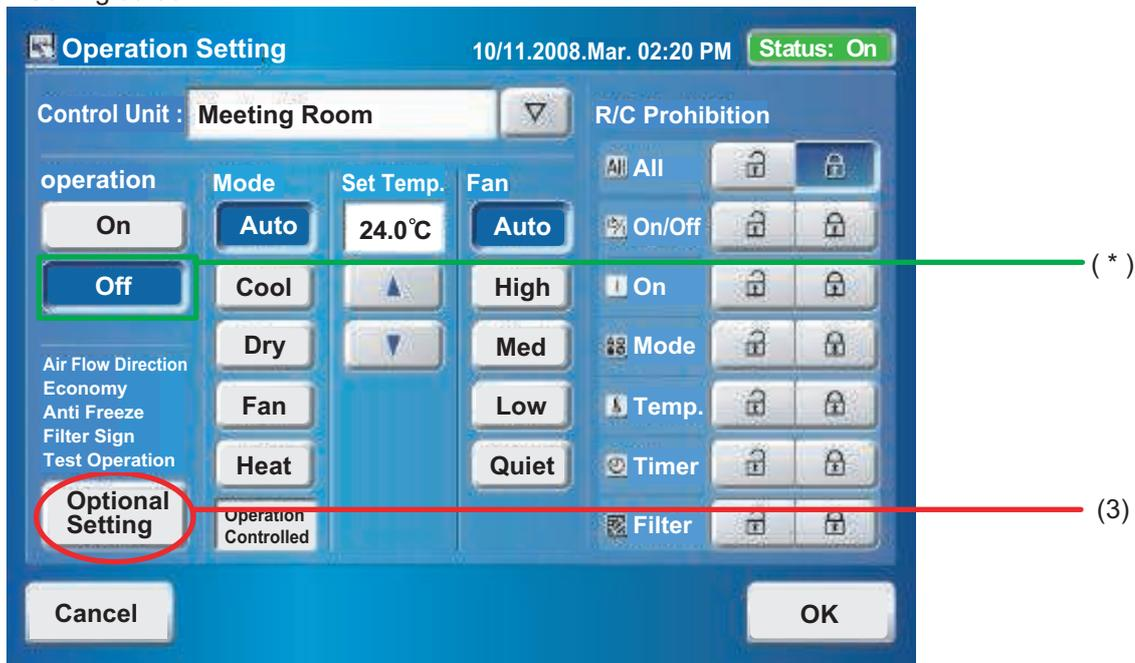
3. Switch to the Details setting screen by pressing "Optional Setting" on the setting screen.
