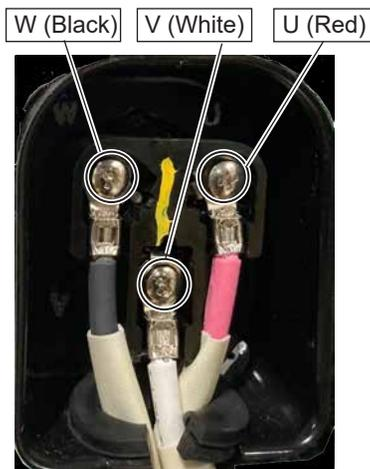
9. Remove the 3 mounting screws of terminal.
