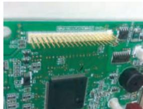
2. Indoor unit transmission PCB install
