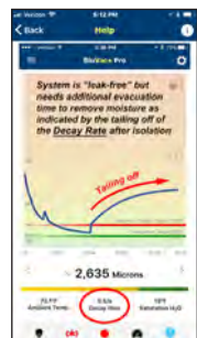
Rise with curving tail indicates tight but wet system that needs further evacuation.
