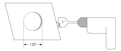
**Step 2:** Wire nut the sensor to cable run between the flush mount sensor and the thermostat or support module. Press the sensor into the 1" hole after the wires are connected.
