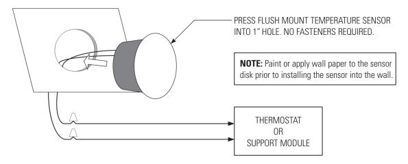
**Step 3:** Wire the sensor to the thermostat or support module. Refer to the instructions provided with these devices for additional details.
