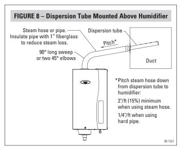
If the dispersion tube must be mounted below the humidifier or if the steam hose needs to run up and over an obstruction, a drip tee with drain trap, Part #4028, must be installed as shown in **Figure 9**. When using a fan pack, install Part #4028 close to the humidifier outlet to help prevent noise from gurgling as shown in **Figure 10**.
