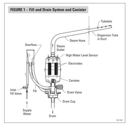
fitted with opening called "Tubelets™". The design of the dispersion tube and Tubelets distribute steam over a wide area in the duct and direct any condensed moisture back into the steam hose. The blower activation function on the ADHC allows the control to turn on the HVAC system blower to maintain the proper RH level even when the furnace or air handler is in stand-by mode. See ADHC installation manual.
