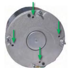
On RESCUE® 5.6" diameter motors lead end blind holes (4) are for mounting on Rheem® and Trane® units requiring grill mount motors. Special screws are provided.
