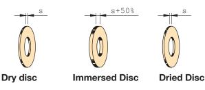
When the system is operating under normal conditions, the discs are immersed and, due to their increase in volume, they close the valve. However, when air is present, the discs dry out and allow the air to vent.
