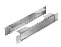
The firestop spacers center vent in 16" O.C. stud space and serve as a firestop at the ceiling level. This is a required component for Type B 2 x 4 and multi-story Type BW installations.
