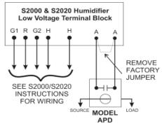
FOR AIR PROVING ON BY-PASS OR FLOW-THRU HUMIDIFIER
