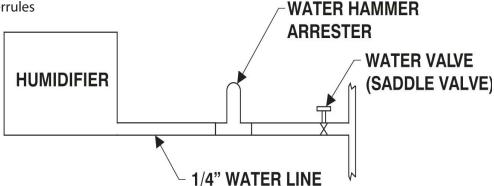
Water Hammer is the term used to define the pounding noise or vibration that occurs in a water line, due to the fast closing action of electric solenoid valves or similar water flow control devices.
