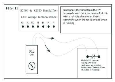
The latest improvement to the Field Controls humidifiers is the new "Airflow Interlock Feature" provided on the low voltage terminal block. Due to popular demand we have made it easier for you to achieve fail safe lockout in the event the fan or blower on the HVAC system does not operate when called upon. A high humidity or airflow proving device is necessary.
