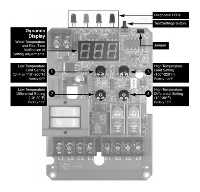
**NOTE:** Be careful not to select overlapping temperature settings. For example: If the HIGH TEMPERATURE LIMIT is set at 190°F with a HIGH TEMPERATURE DIFFERENTIAL set at 20°F, then the LOW TEMPERATURE LIMIT needs to be set at 170°F  $(190^{\circ}F - 20^{\circ}F = 170^{\circ}F)$  or below.
