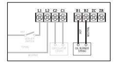
**STEP 3** Connect the burner circuit to **B1** and **B2.** (B2 is neutral.)
