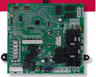
**Two-Stage 21V51D-751** Replaces Carrier/ICP equipment brands Blower Motor Types – PSC, Variable Speed and ECMx with 120V Ignition
