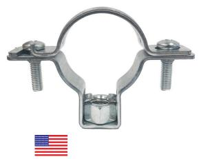
**Galvanized Split Ring Hanger** Used to suspend black iron pipe from joists, steel beams, wooden rafters, or walls. They can be used in both vertical and horizontal applications.
