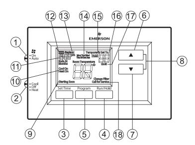
Whenever "Replace" appears in the display, new premium brand AA alkaline batteries should be installed. If the house will be unoccupied for an extended period and either "To r" Replace" is displayed, install new batteries before leaving.
