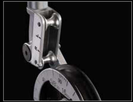
Stainless steel rollers reduce friction against the tube.
