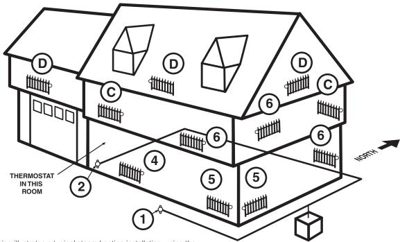
The above drawing illustrates a typical steam heating installation, using the correctly sized Gorton Vapor Equalizing Valve on each radiator to make all rooms heat evenly and comfortably. The use of a No. 2 Gorton Air Eliminator at the end of the long main, and a No.1 Air Eliminator at the end of the short main is also indicated.
