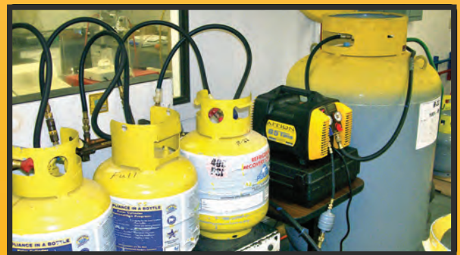
Below: G5Twin used daily in a reclamation facility for tank to tank transfers
